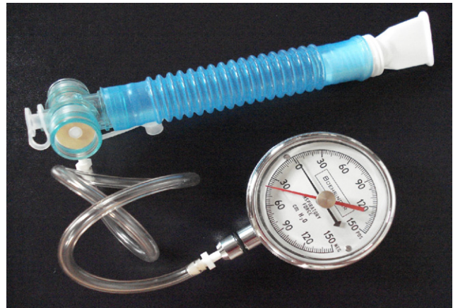
Fig 1. The Boehringer High Pressure Inspiratory Force Meter.
